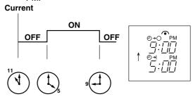
**NOTE**: If the main power is turned OFF or a power failure occurs while ON/OFF timer is active, the timer setting is cancelled. As these models are equipped with an auto restart function, the air conditioner starts operating with timer cancelled when power is restored.
