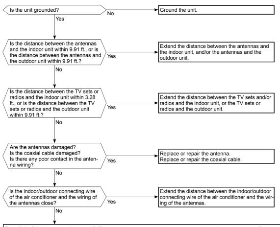
Even if all of the above conditions are fulfilled, the electromagnetic noise may enter, depending on the electric field strength or the installation condition (combination of specific conditions such as antennas or wiring). Check the followings before asking for service.
