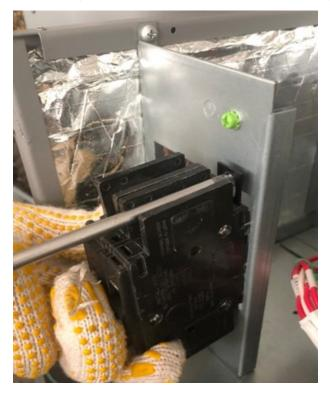
7. Connect the electric heater terminal
